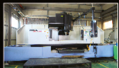
Machining center : CNC VM960L(2600*950mm)
